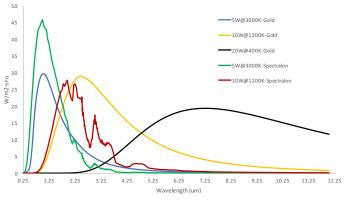
COLOSUS extends the radiance possibilities from the VIS to the LWIR with a variety of sources, spheres and blackbodies for complete calibration of your instruments. Select, combine and tune your calibration sources to match the dynamic range and spectral performance of your instrument.
