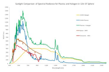
Halogen spectrums are the industry standards, but often represent problems for advanced instrumentation as they are "red-weighted" sources leaving your test lacking in blue-weighted solar spectrums. COLOSUS systems add innovative plasma and xenon sources so you can test with tuneable spectrums actually resembling solar reflective target spectrums and levels. Test as you Fly and Fly as you Test for highest accuracy.
