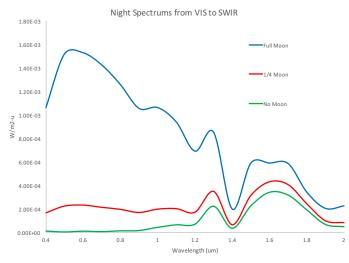
Use night sky spectrums and levels for instrument verification. Combine sources or filter sources to suit the test needs. Today's night vision systems are challenging not only visible ranges but extending to the SWIR for enhanced performance and sensor fusion. COLOSUS dynamic range can cover day levels and night levels continuously in one system.
