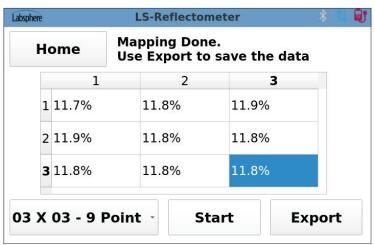
Target mapping mode simplifies reflectance mapping with two mapping options; 3 X 3, nine point maps, and 5 X 5, 25 point maps.
