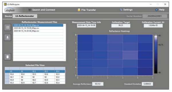
RefAquire works with the reflectometer hardware in real time over USB to provide file transfers, file maintenance, and data visualization. RefAquire's reflectance heatmap creates a data visualization tool that provides a fast and efficient way to evaluate reflectance data with a quick glance.
