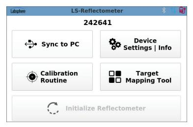
The Reflectometer's user friendly touchscreen interface puts device calibration, data transfer to external PC, target reflectance mapping, and single scan measurements at your fingertips.
