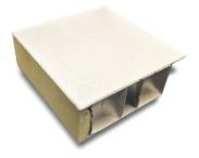
Commercial Targets are 18.5 - 25.4 mm thick and consist of an aluminum honeycomb network sandwiched between two sheets of aluminum. The material design provides a mechanically flat, rugged, and lightweight target backing solution available in four standard target sizes; 0.5 m x 0.5 m, 1.0 m x 1.0 m, 1.5 m x 1.5 m, and 1.2 m x 2.4 m, with or without mounting.
