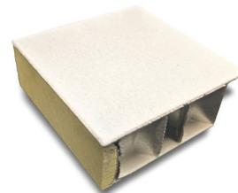
Lidar Targets are 18.5 - 25.4 mm thick and consist of an aluminum honeycomb network sandwiched between two sheets of aluminum. The material design provides a mechanically flat, rugged, and lightweight target backing solution available in four standard target sizes; 0.5 m x 0.5 m, 1.0 m x 1.0 m, 1.5 m x 1.5 m, and 1.2 m x 2.4 m, with or without mounting.
